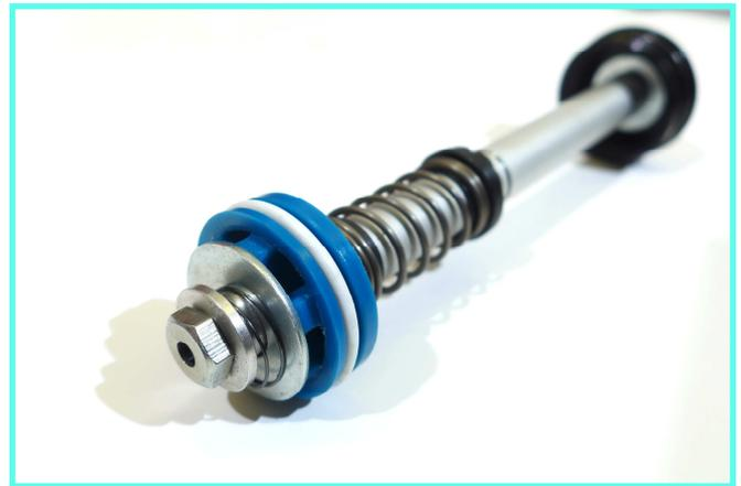
**Low a High speed compression controls the speed at which the fork compresses.**
